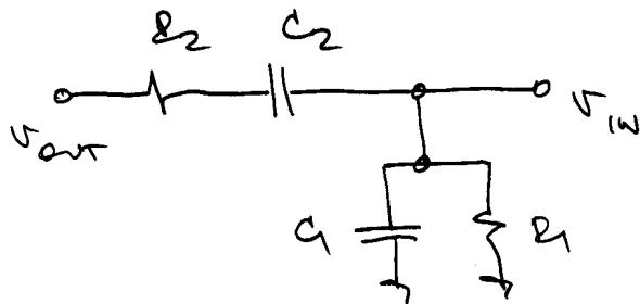
$$\beta(s) = \frac{V_{in}(s)}{V_{out}(s)}$$
